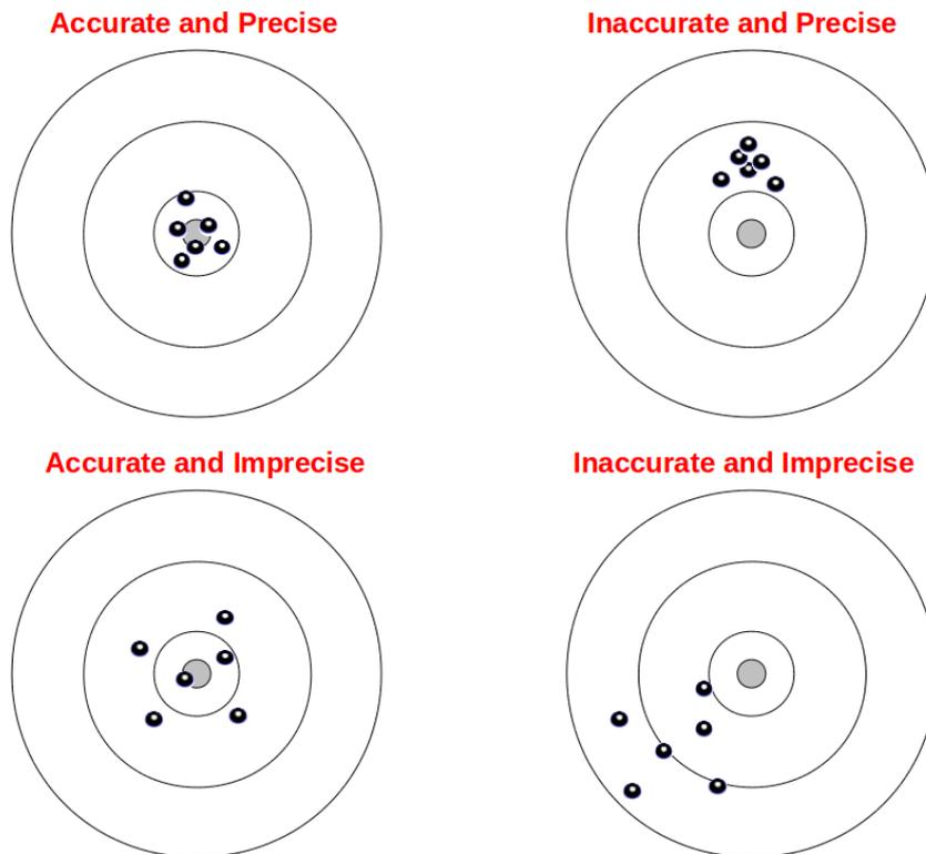
Aim of Gage R&R is to assess the **precision** of measurement system.
